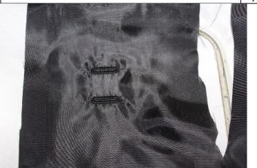
If you want to make a ribbon to pull out the phone. Make loops on the sewing machine on the lining fabric.
