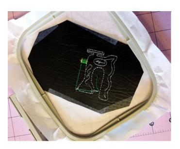
4. Stitch through the various color changes up until the last one. These are the details of your design. Before stitching the last color, remove the hoop from the machine.
